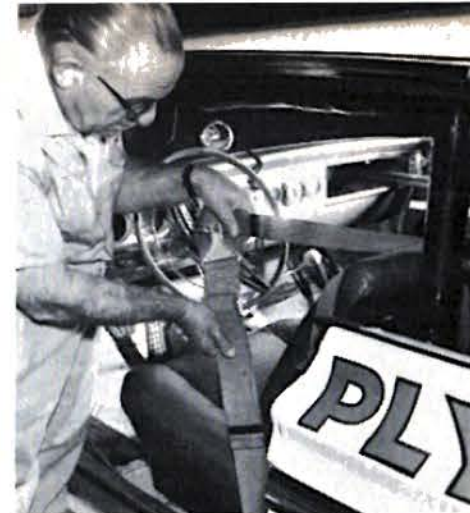
Norm points out the huge ports in the new Super Commando hemi heads. Note the special pistons used in all hemi engines. Manual gas shutoff valve handle mounts to the right of the shift lever. Big fire extinguisher rests in place of the passenger's bucket. To comply with Bonneville safety regulations, Norm installed a three-inch wide seat belt and a two-inch wide harness.
