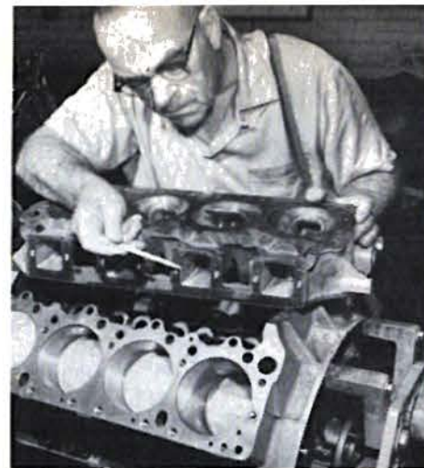
Norm points out the huge ports in the new Super Commando hemi heads. Note the special pistons used in all hemi engines. Manual gas shutoff valve handle mounts to the right of the shift lever. Big fire extinguisher rests in place of the passenger's bucket. To comply with Bonneville safety regulations, Norm installed a three-inch wide seat belt and a two-inch wide harness.
