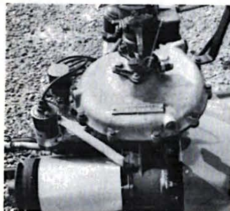
Graham centrifugal supercharger is used with a Ford 97 two-barrel carb for the intake system. Carb linkage is hydraulic.
