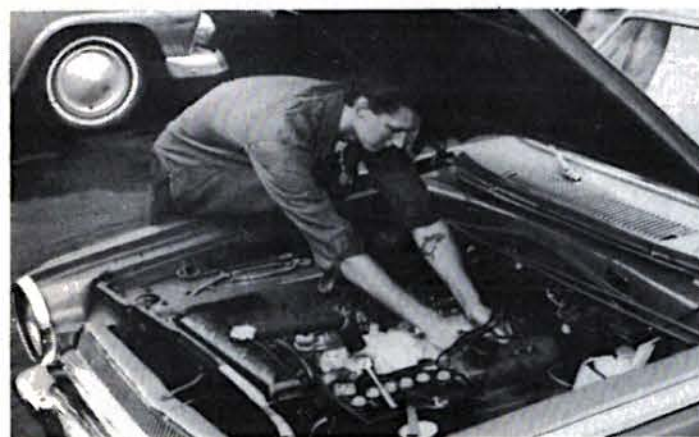
S&P technician, left, installs the single quad manifold on the test Dart. Comparison shot, below, shows the factory two-barrel setup flanked by Offy single and dual quad manifolds.
