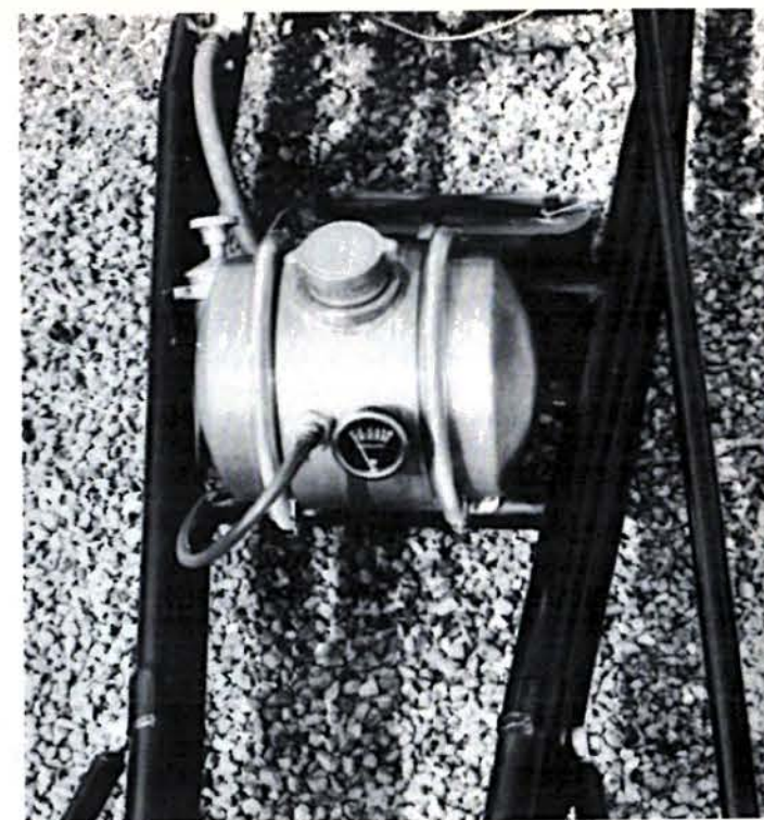
Small aluminum fuel tank and pressure pump mount up front. Team members (below) demonstrate just how light this dragster is. Ultra-lightweight rail tips scales at 550 lbs!
