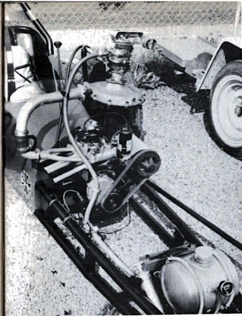
Blown '46 Fiat displaces 30.5 cubes. Aluminum head was milled .080-inch for extra power. Pistons are stock.
