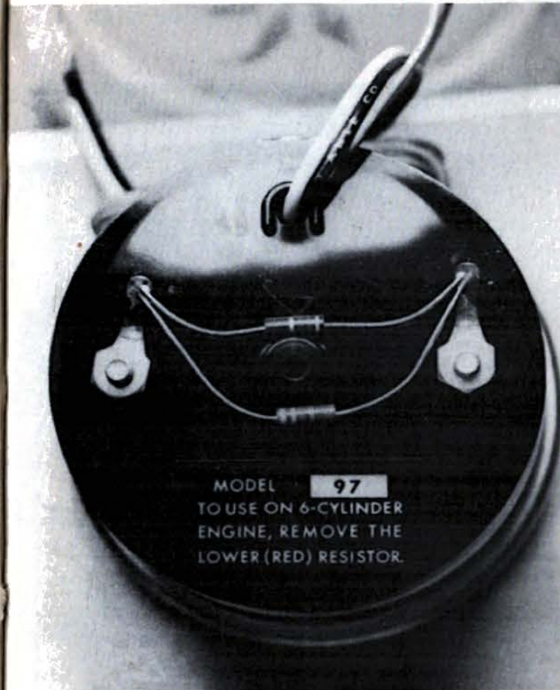
By simply removing the red resistor from the rear of the large Model 97 tach, you can install an Eight-cylinder unit on a Six-cylinder engine. Installation is simple.
