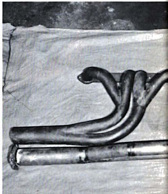
Current hemi headers (above) use cast adapters to reduce cost. Interference headers (right) do not provide peak performance, but are fine for the street.
