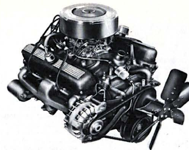
Optional 10.5-1 four barrel 273 engine is available on all '65 Darts. Goodies include a hot cam, special pistons, quad and a chrome dress-up kit.
