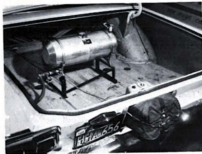
Another safety feature is the special five-gallon gas tank bolted to the trunk floor. Note the chute release cable and beefy fuel lines. Both cars are equipped with drag chutes and legal California street registrations!
