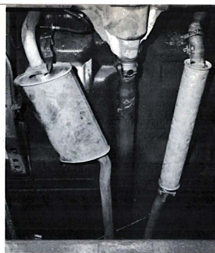
Duals must be fabricated for this engine, as the factory only offers a single setup. Stock headers are restrictive.
