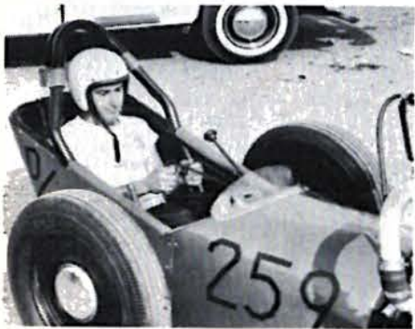
Roll bar offers adequate driver protection in case of spill. Note the long shift lever and abbreviated plexi windshield.
