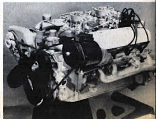
Streamlined Catalina 2+2 with buckets, aluminum wheels and 421 mill is Pontiac's top performer for '65. New Olds Hydro has a variable vane stator. Controlled shifts make it ideal for competition use. Buick 425 dual quad mill is available on all Riviera, Electra and Wildcat models. Aluminum components are used to keep the weight down to a minimum. It's a hot one!
