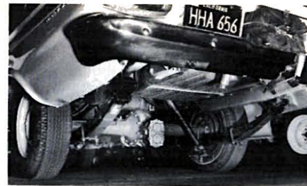
Halibrand quick change center section and Police springs and shocks bring up the rear. Front suspension is stock. Norm is shown with the car that will run in B/SC. Norm tuned 195.97 mph with a wedge last year.
