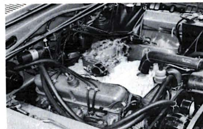
Offy single quad AFB setup is ideal for the guy who wants more punch, but doesn't want to go the cam route.
