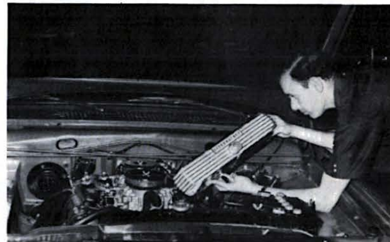
Offy makes finned aluminum valve covers for the 273 Charger mill. Note the neat chrome air filters on the quads. Clutch disc, below, is available with a pressure plate from Hayes.
