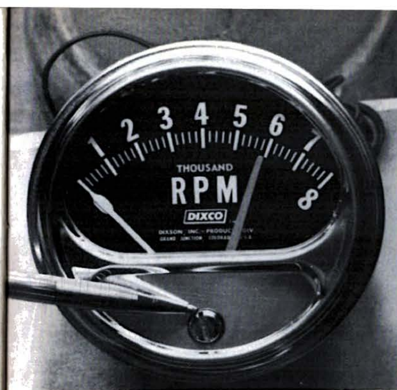
An adjustable redline or shift pointer is a must if you want to get the most from each shift. Shift points vary with transmission, rear end gear, and tire changes.
