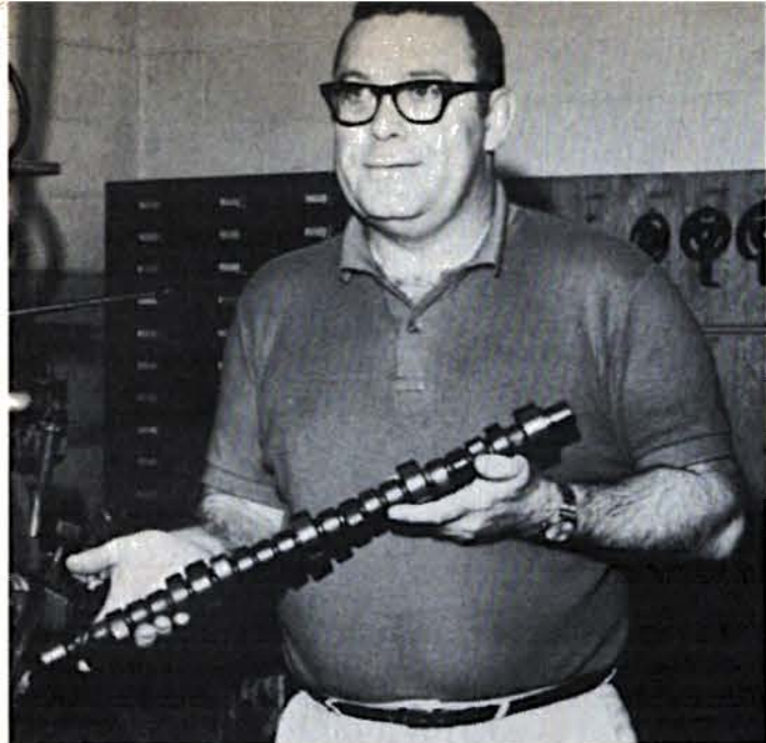
Racer Brown displays his latest (ST-14-street-strip) .485-inch lift, 266-degree duration, solid lifter 273 Charger cam.
