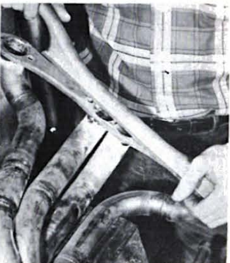
A wide-tooth file can be used to show up high spots and straighten the flange.
