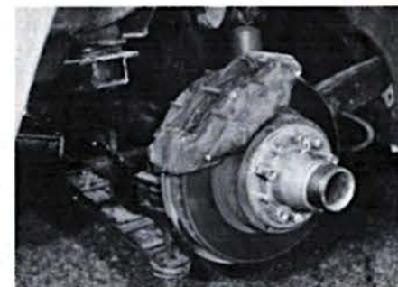
'Vette discs have built-in drums for parking brakes. Action is positive.
