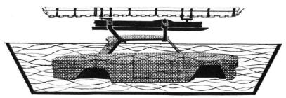
String up a conveyor system to deep-dip car bodies—right to the roofline—in a monster tank containing 12,000 gallons of rustproofing primer paint. (Most other car makers settle for spray-on rustproofing.)
