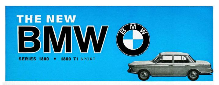
"A UNIQUE DEVOTION TO TECHNICAL PERFECTION AND DETAILED CRAFTSMANSHIP!" FOR EXAMPLE: 124 H.P. (OPTIONAL EQUIPMENT AVAILABLE UP TO 170 H.P.) WITH OVERHEAD CAMSHAFT AND INCLINED VALVES. INDEPENDENT 4 WHEEL SUSPENSION WITH MAC PHERSON-TYPE SPRING LEG FRONT AXLE AND LONGITUDINAL SWINGING REAR WHEELS. 4-SPEED PORSCHE-TYPE SYNCHROMESH GEARBOX. POWER ASSIST BRAKES WITH DISCS IN FRONT.
