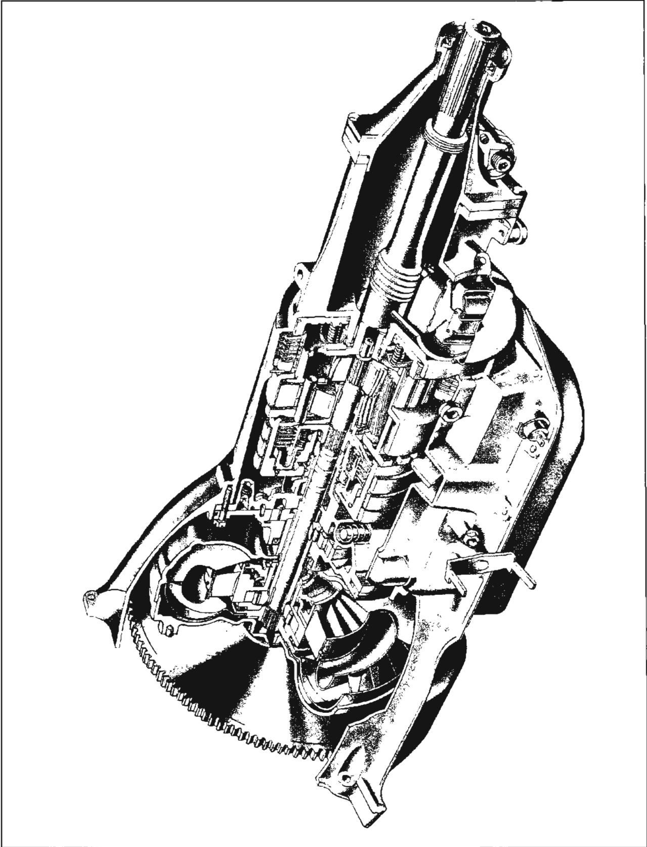
Figure 5-9—Cross Section of Transmission
