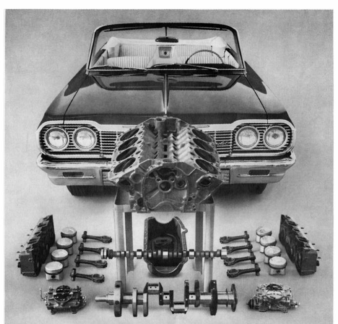
YOU LIKE PLAYING WITH BLOCKS, TRY THIS. With Chevrolet's Turbo-Fire 409 V8\* block you can build to great heights. Say, 340 hp. 400 hp. Or, with the ingredients shown here, 425 hp. All three use the same block. Looks like the Rock of Gibraltar with 409 cubic inches of tunneling punched in it.
