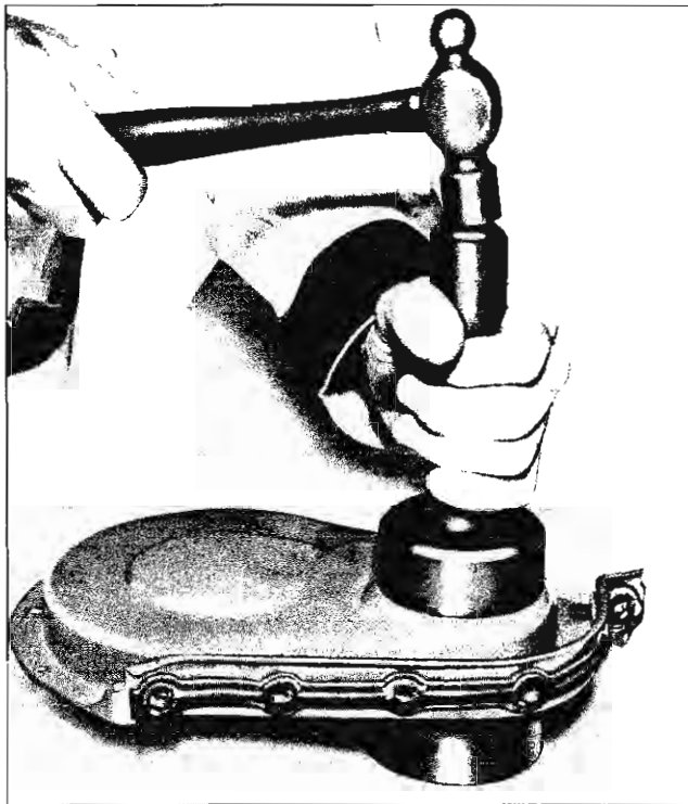
Fig. 29—Installing Timing Gear Cover Oil Seal
