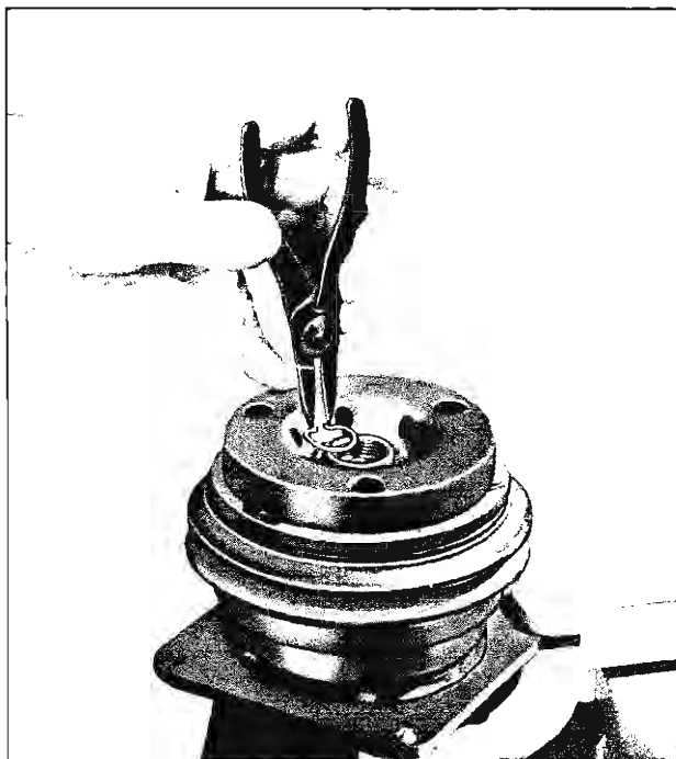
Fig. 30—Removing Coil Housing Retainer Ring
