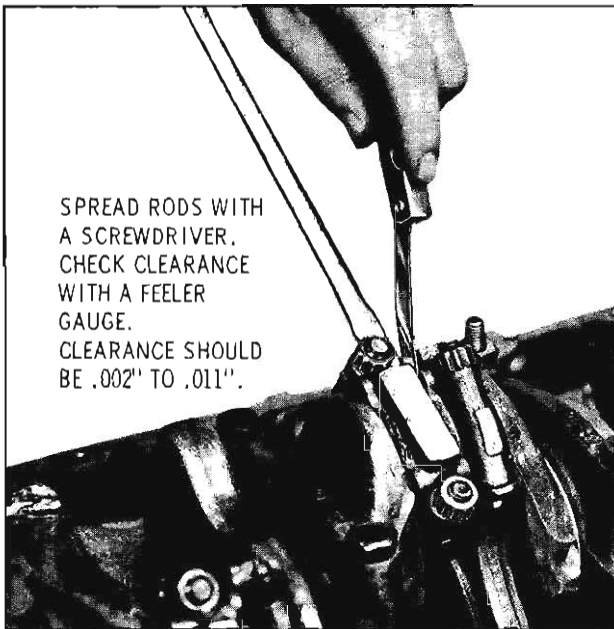
Fig. 3-428 Connecting Rod Side Clearance
