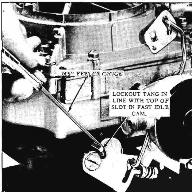
Fig. 4-171 Secondary Throttle Lockout Adjustment
