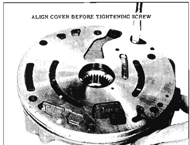
Fig. 6-57 Installing Pump Cover
