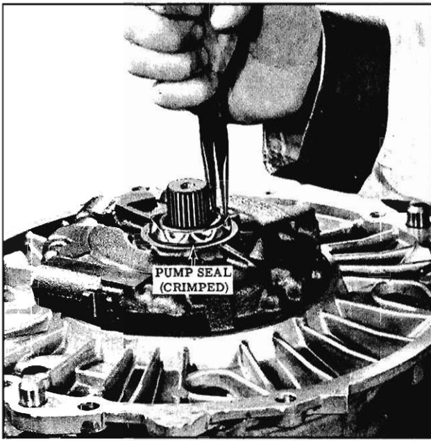
Fig. 6-31 Removing Oil Pump Seal
