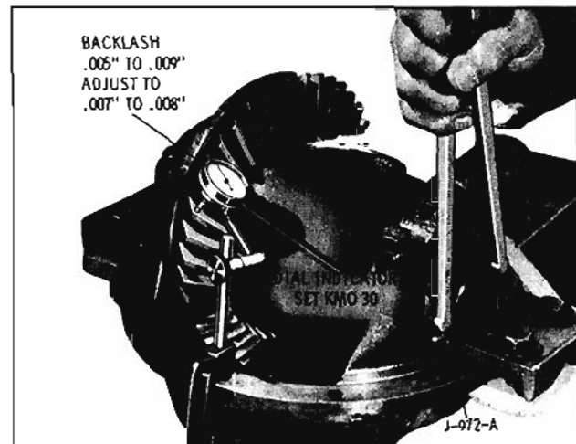
Fig. 10-36 Adjusting Backlash
