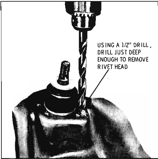
Fig. 9-1248 Drilling Upper Ball Joint Attaching Rivets
