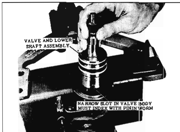
Fig. 8-68 Installing Valve and Lower Shaft Assembly
