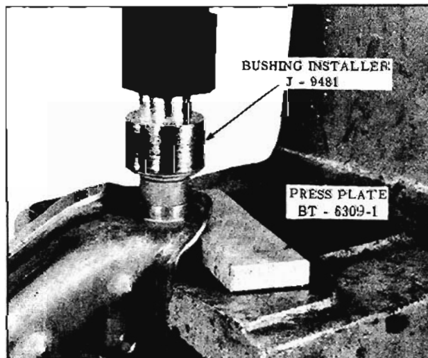
Fig. 9-23 Installing Pivot Shaft Bushing
