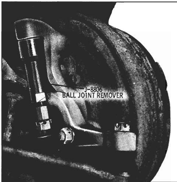
Fig. 9-111 Disconnecting Ball Joint
