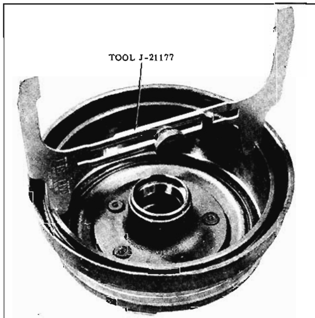
Fig. 11-4 Checking Brake Drum
