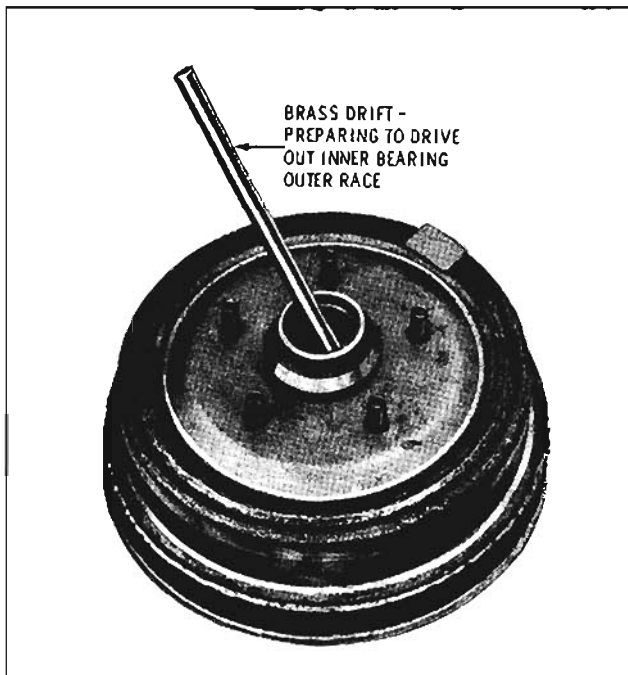
Fig. 9-105 Removing Wheel Bearing Races
