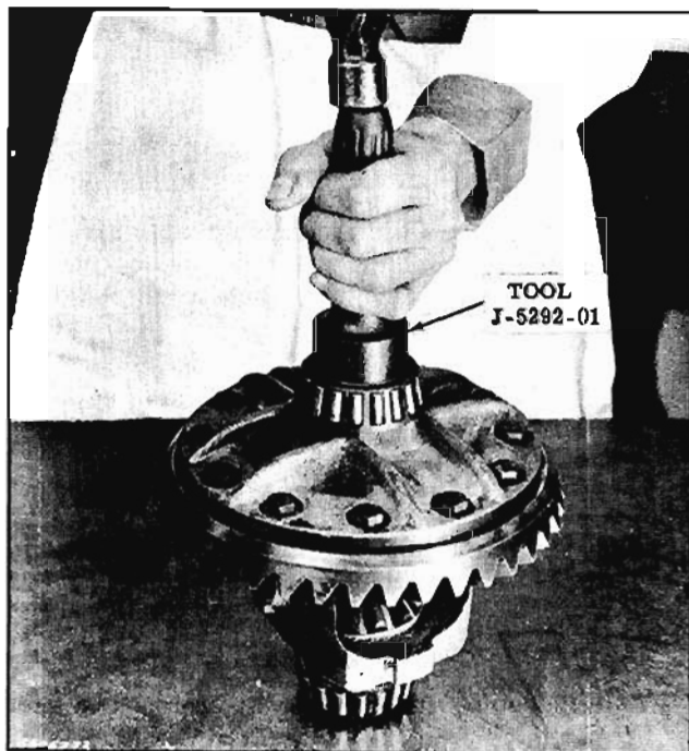
Fig. 10-26 Installing Side Bearings
