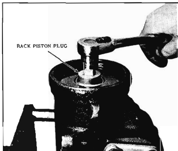
Fig. 8-45 Removing Rack-Piston Plug
