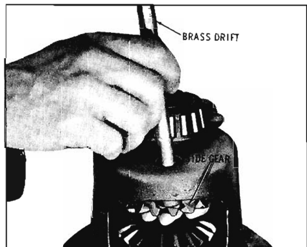
Fig. 10-40 Removing Side Gear
