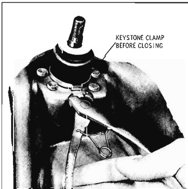
Fig. 9-123A Installing Ball Joint Seal
