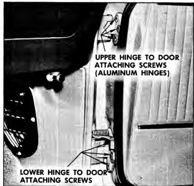
Fig. 16-329 Front Door Hinge Attachment
