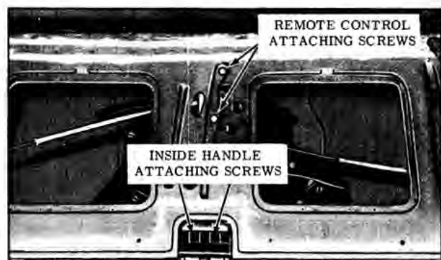
Fig. 16-221 Remote Control Removal
