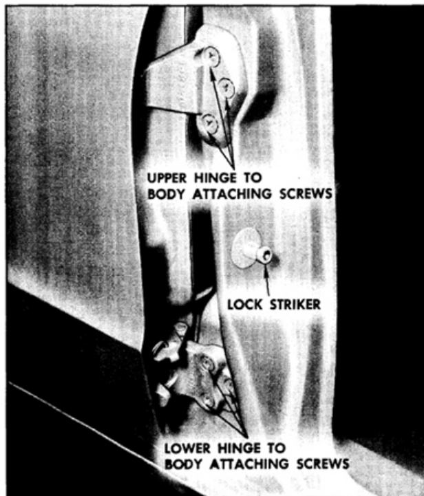
Fig. 16-350 Rear Door Hinge Attachment
