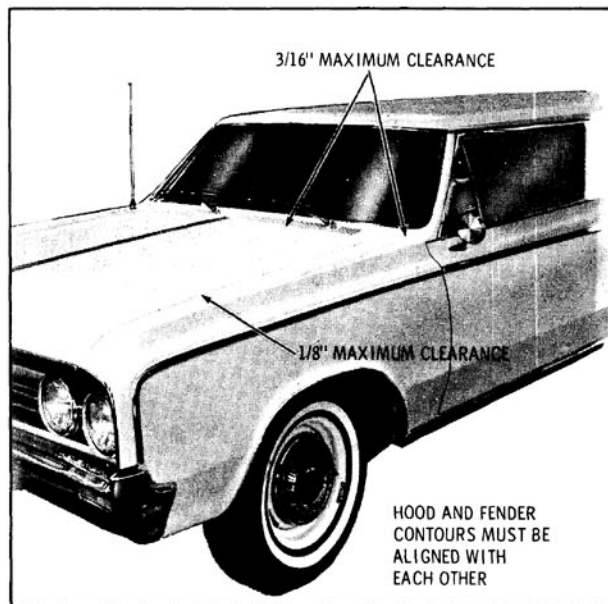
Fig. 15-110 Hood and Fender Clearances
