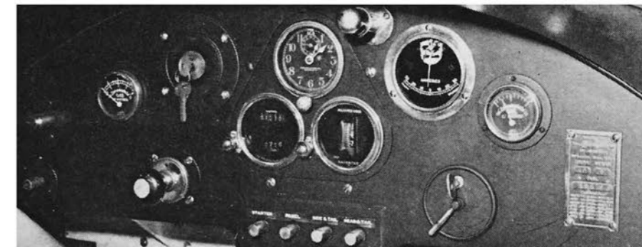
AUTHENTIC INSTRUMENT panel includes original Locomobile gas and oil gauges, speedo and odometer, push-switches and ignition switch.
