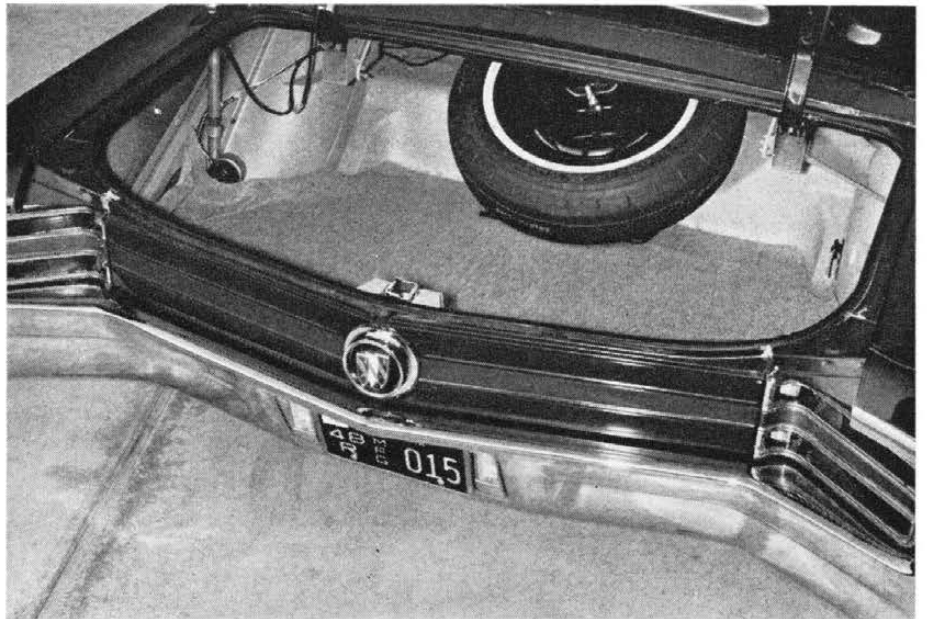
WIDE, WIDE trunk has flat floor and high lift-over height, but capacity is tremendous. Electric antenna mechanism is at left.
