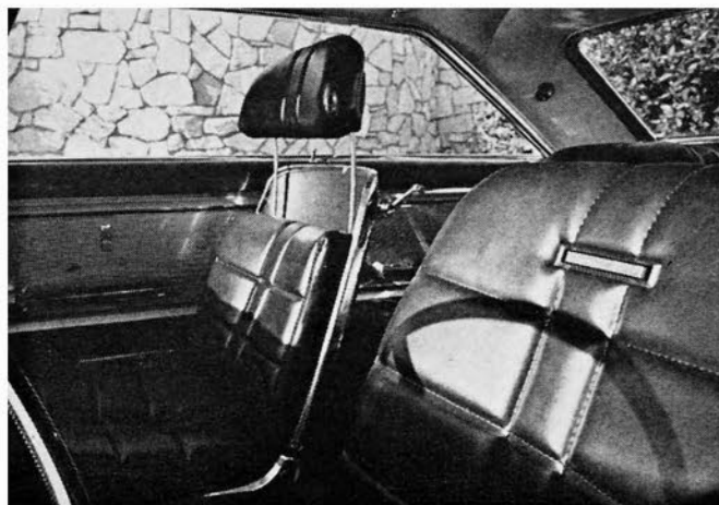
PARK LANE bucket seats are similar to Thunderbird's, complete to headrest sliding up on stalks.
