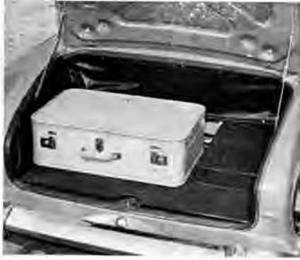
LEFT - Trunk compartment is surprisingly adequate; beneath floor, spare tire, tools and 12-volt battery. Convertible top is manually operated.
