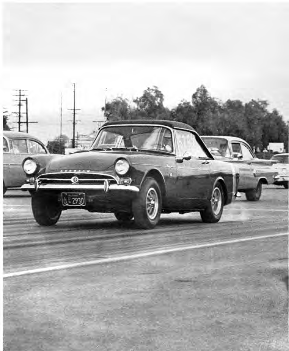
Second test car carried hop-up goodies; 4-bbl, Cobra cam, mag wheels, etc., ran 15-second e.t.'s "box stock" at Pomona drags with Gary McKeand driving. This one should be real good on quarter when "uncaged" through strip tuning.
