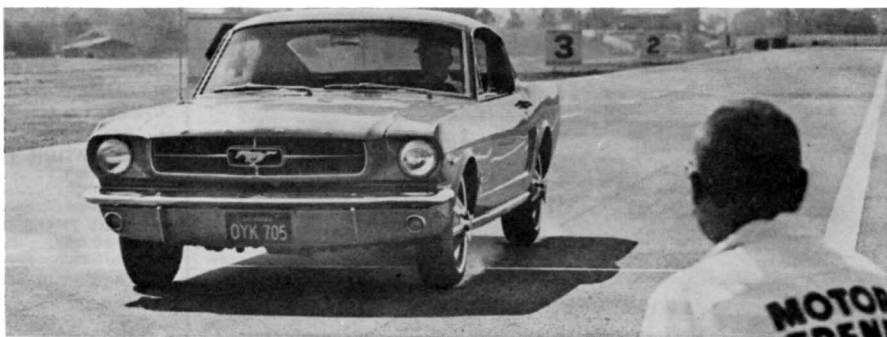
We had to work to lock up all four wheels during panic stops, but it was possible. Combination of discs and drums is a great improvement, always gives fast, straight stops.
