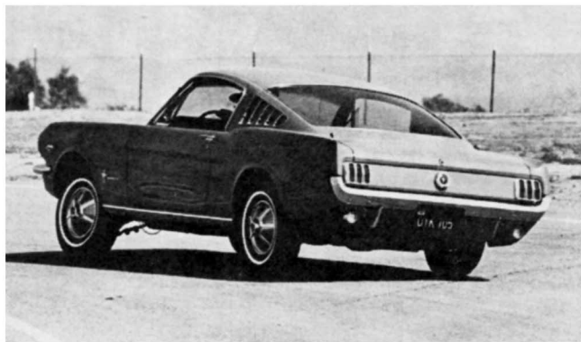
Mustang's side louvers serve as air-exhaust vents to get rid of stale air. Fastback design limits driver's view to the rear.
