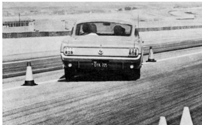
With four aboard, our Mustang charged through pylon gate with only slight amount of body lean. Added weight aided control.
