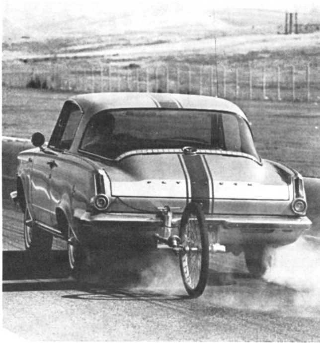
Plymouth's combination of 235-hp V-8, Sure-Grip differential with 3.55 gears, and four-speed gearbox add up to a hot performer.
