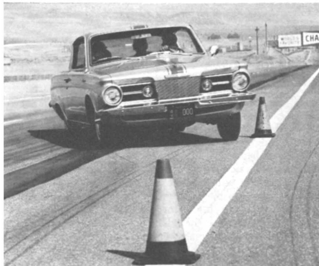
Heading through pylon gate at 35 mph with four aboard, the car showed only slight body lean, actually handled better with load.
