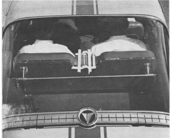
Tinted rear window's heat-absorbing qualities eliminate 33% of sun's spectrum, remove 45% ultraviolet, 35% infra-red rays.
