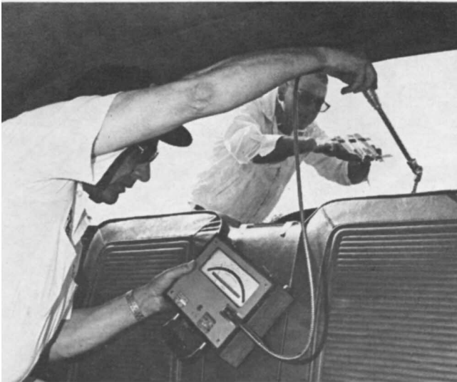
Cruising at 60 mph with vent panes and air vents open, temperature at back of seat registered 98° vs. 82° at window.
