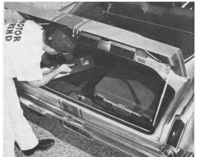
With panel closed, there's room in trunk for suitcases. Twin exhaust vents under lid let stale air out of passenger area.
