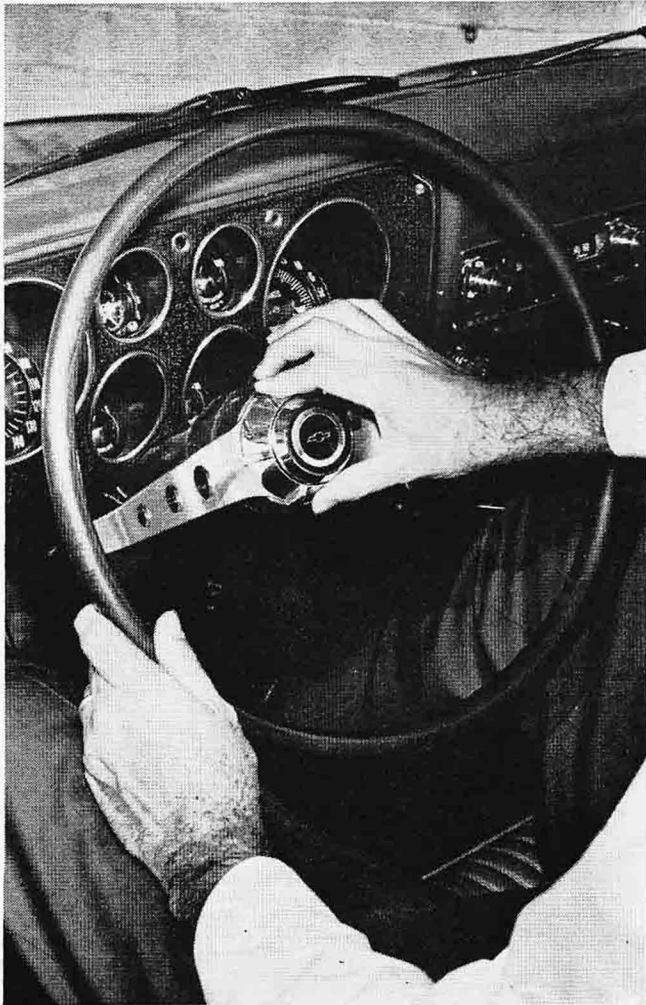
Telescoping steering wheel can be adjusted to any position in a three-inch range. Cog at horn button loosens and tightens it.
