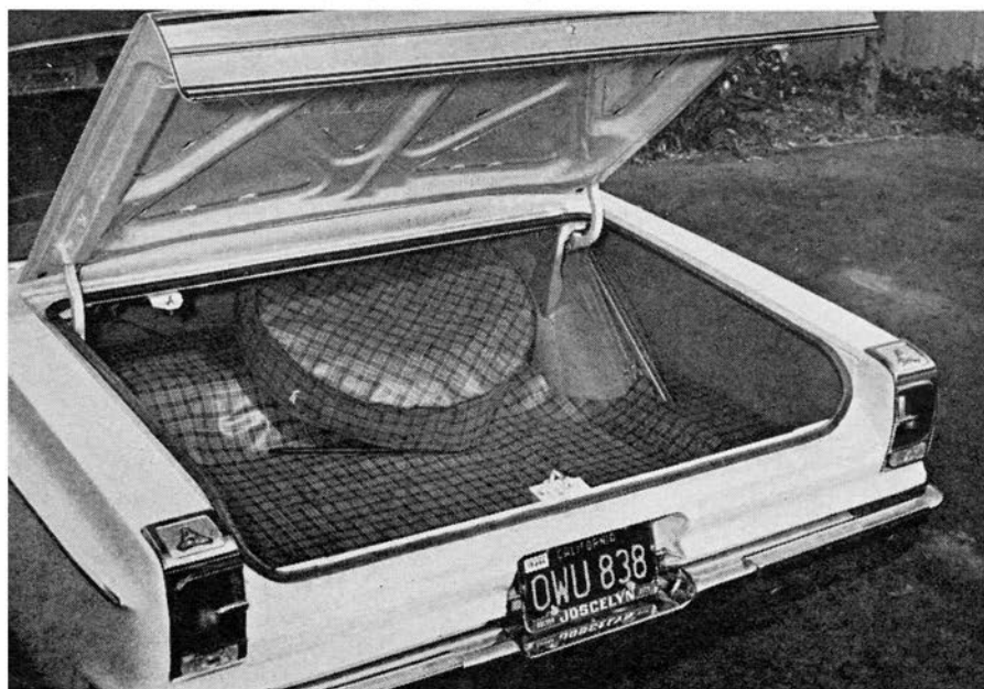
BIG TRUNK would be larger with horizontally mounted spare tire. Fuel filler cap is hidden behind spring-hinged license plate.
