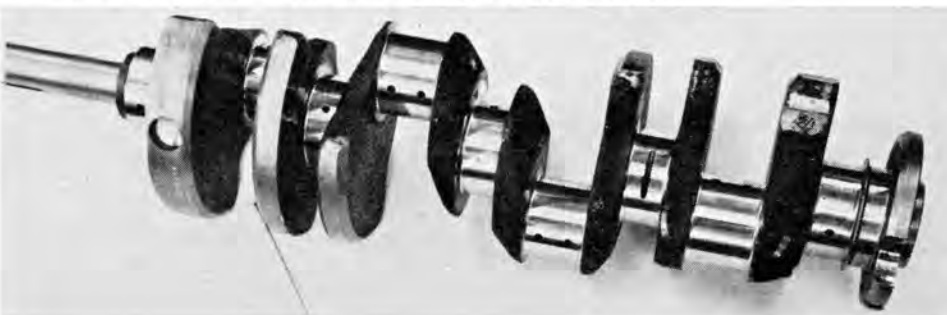
CRANKSHAFT CHANGES for increased high rpm durability of 427s included cross-drilling of crankpins and main journals, spacing main journal oil holes 180° apart.
