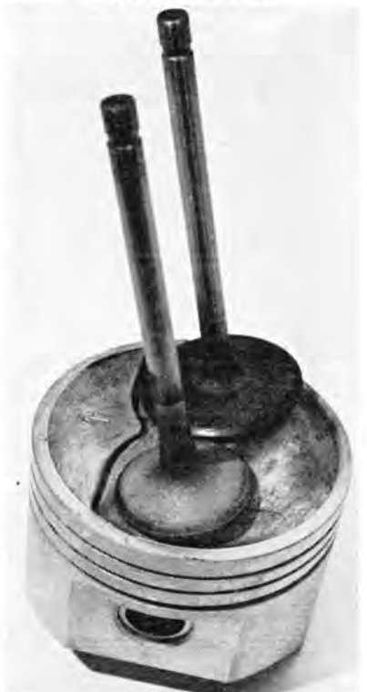
HIGH compression pistons require indentations for valve clearance.
