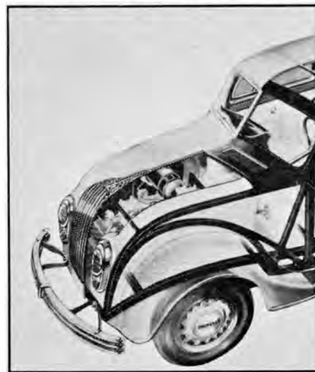
CHRYSLER Airflows were designed as full-unit bodies but had light frame superstructure.
