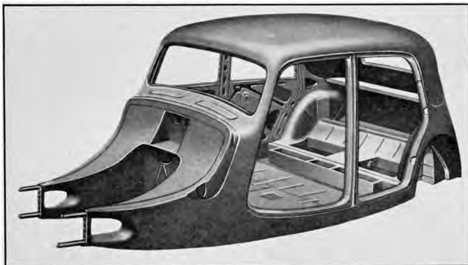
CITROEN PUT this unit body into production in 1934, continued it until 1954. Note heavily braced cowl, roof and floorpan areas.
