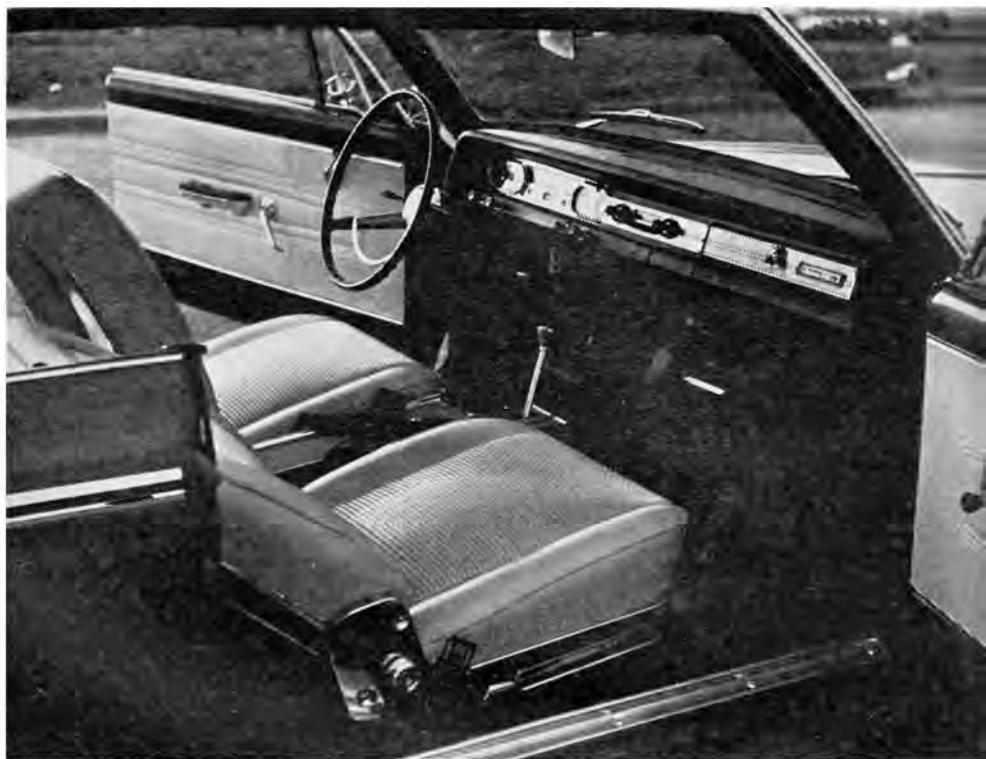
RECLINING BUCKET seats have cross-ribbed cushions but are little changed from last year. Stout, stubby shift lever for automatic juts up from console.
