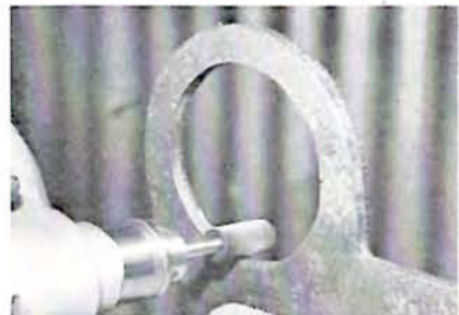
A hand-cut cylindrical rotary file is ideal for smoothing edges of flame-cut parts on that car. A Black & Decker 1/4" Holgun drill spins file at 2500 rpm's.
