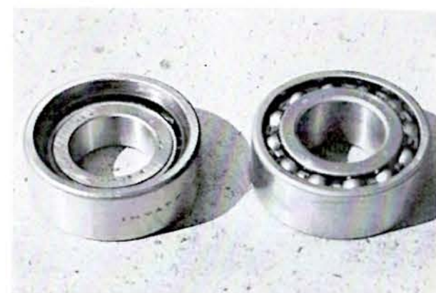
The bearing on the left is a roller type for the rear. Double row ball bearings, right, are used in front end plates. SAE 30 engine oil is recommended for lubrication.
