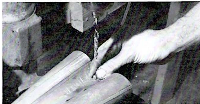
A stock retaining pin, \frac{7}{8} " from the rotor end, is backed up another pin in a different channel. A \frac{1}{4} " hole is drilled, then reamed with a taper reamer until the pin will drop into the hole, allowing the head to protrude only \frac{1}{16} inch.
