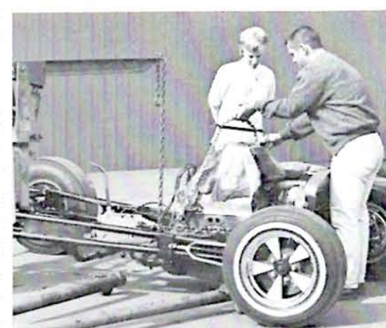
After taking delivery of the Dragmaster Streetster chassis, Billy bolted together the front and rear end components and got the thing on wheels before installing the engine. Wife Jeanie helps when needed.
