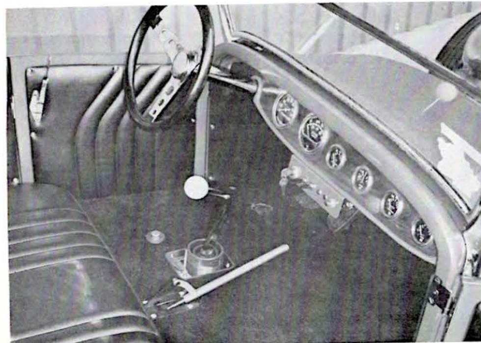
Below — A fibreglassed wooden dash helps highlight the black Naugahyde and carpet interior. Special opening doors are all wood reinforced, body is channeled over the frame 3 inches. Headlamp dimmer switch is to left of shifter, all other electrical controls are on plate under dash.
