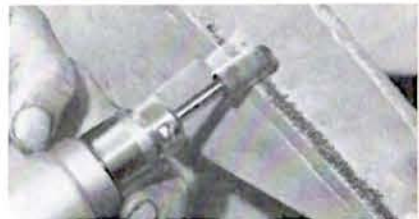
When dressing down an aluminum weld or reshaping soft, non-ferrous metals, a ground bur is the best choice since it will not clog. Maintain even movement.
