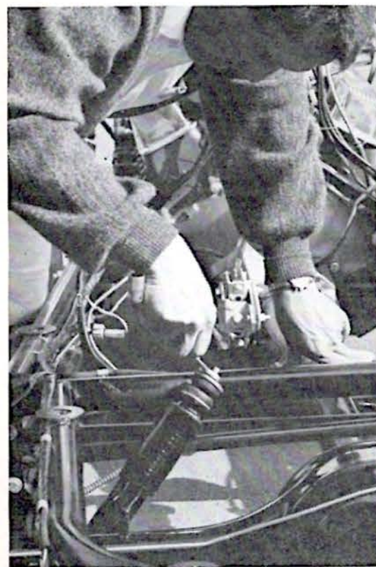
With everything on the chassis in place, Kellison fiberglass body was dropped in position. S-W gauged dash and Simca emergency brake handle, steering installed.
