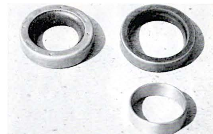
At left is a stock leather-lined seal while on the right is a rubber replacement seal with metal sleeve. The sleeve slips onto the stock shaft, improving sealing, since it is likely worn.
