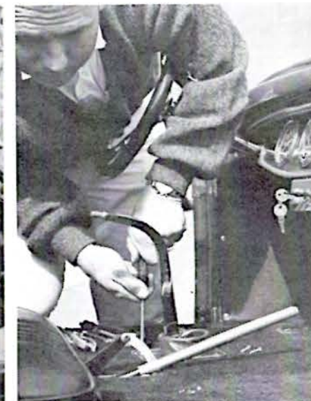
With everything on the chassis in place, Kellison fiberglass body was dropped in position. S-W gauged dash and Simca emergency brake handle, steering installed.
