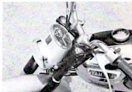
Speedometer and headlight reside in single nacelle. Entire unit tilts for easy headlight adjustment by loosening bolts.
