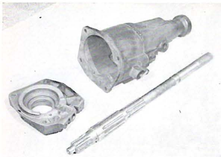
The R-11 overdrive unit uses a special adapter plate, at left, when used with most transmissions. The special tailshaft is about 25½ inches.
