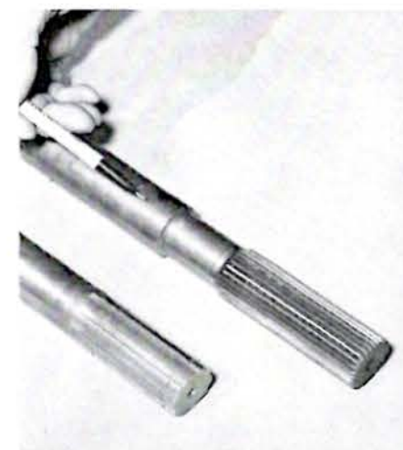
Stock Ford 4-speed tailshaft, top, has different splines than needed, is about 2 inches too long. Include Ford tailshaft when ordering to avoid core charge.
