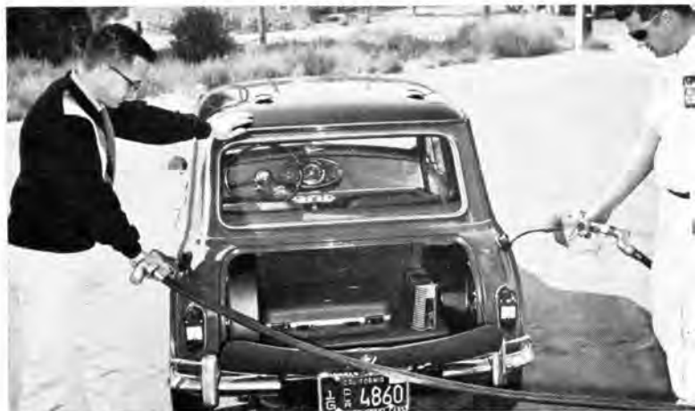
Mini's twin tanks hold 6 gallons apiece. At over 30 mpg, that's a long, long way. Trunk is handy if not spacious, while hanging deck lid allows double loads if tied down well.
