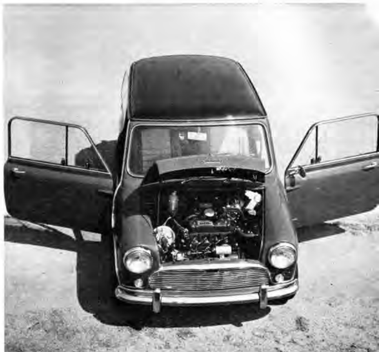
No mistake here — engine sits broadside, leaving amazing leg room inside. Sliding windows are mixed blessing. Doors open wide for easy entrance and exit; have big, handy storage bins.
