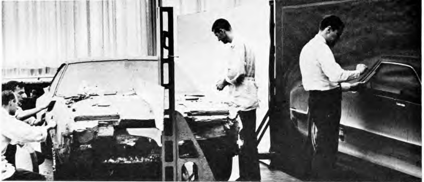
TRAINED EYES OF CLAY MODELERS TAKE SHAPES DIRECTLY FROM FULL-SIZED RENDERING, WHOSE LINES ARE CHANGED ALMOST DAILY BY VIP'S.
