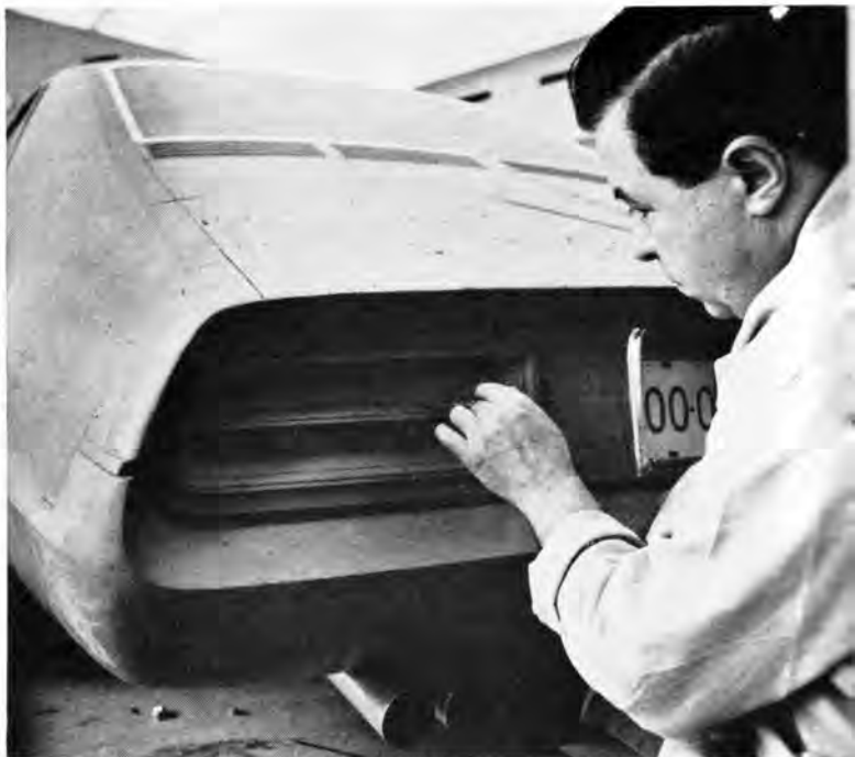
Clay modeler details prototype Toronado. These craftsmen work to .01-inch accuracy with special material costing 37¢ a pound.
