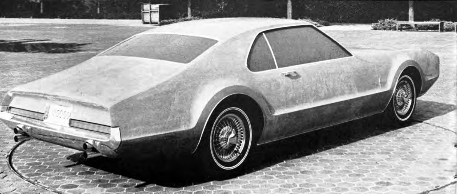
NOVEL EXHAUST TREATMENT FAILED TO MATERIALIZE ON PRODUCTION VERSION, BUT THE VENTLESS FRONT WINDOWS WERE FINALLY ADOPTED.
