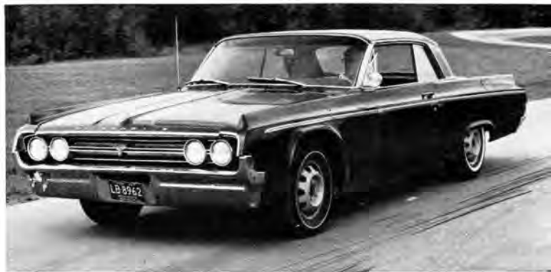
Oldsmobile engineers disguised Toronado running gear under cobbled Dynamic 88 body. Sharp teen-agers still recognized it.
