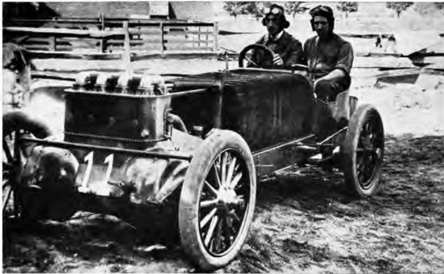
(ABOVE) America's greatest fwd pioneer was Walter Christie, here poised at the wheel of his 1905 racing car. Crosswise 4-cylinder engine mounted atop enclosed drive system, with a huge radiator lying exposed just in front of the tiny cockpit.
