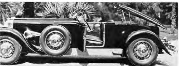
One-off, Miller-engineered, boat-tail speedster used blown V-8 (325 hp) and fwd. Total height with top up was 4 ft., 10 ins.
