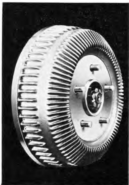
Large, finned, cast-iron drum brakes do creditable job of stopping 4800-pound car.
