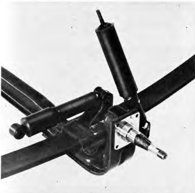
Extremely simple rear suspension consists of 2 usual shocks, plus 2 for braking wind-up, hat section axle, single-leaf springs.
