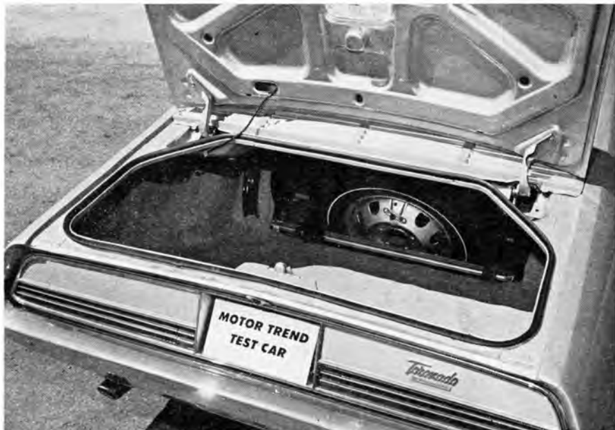
Spare occupies space normally taken by differential hump in conventional cars. Despite truncated rear styling, Toronado has roomy trunk. Deck lid's counterbalanced with springs.
