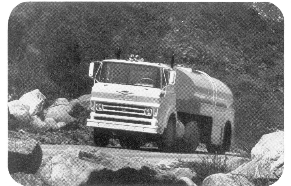
TILT CAB models are only 72 inches from bumper to back of cab to keep overall length at a minimum. Cab tilts forward for easy maintenance access.
