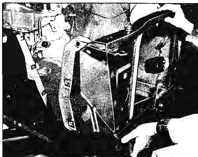
Fig. 32—Removing Radiator Support from Vehicle
