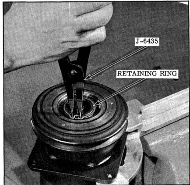
Fig. 14-87 Removing Pulley Retaining Ring
