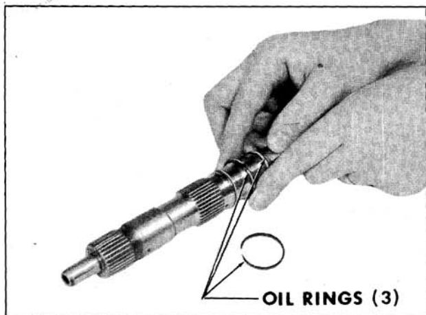
Fig. 6-512 Installing Oil Rings
