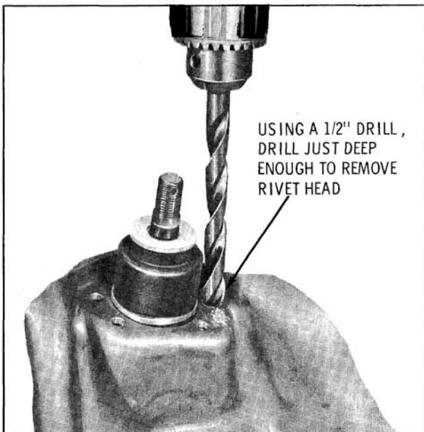
Fig. 9-129 Drilling Upper Ball Joint Attaching Rivets
