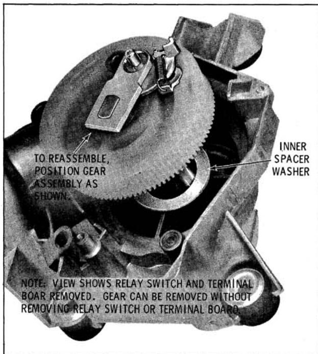
Fig. 13-189 Removing Gear
