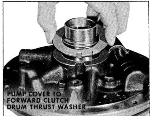
Fig. 6-508 Installing Selective Washer
