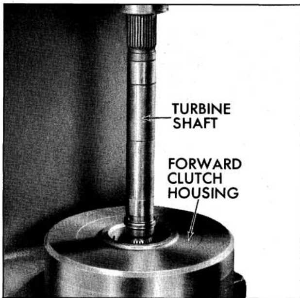
Fig. 6-144 Installing Turbine Shaft
