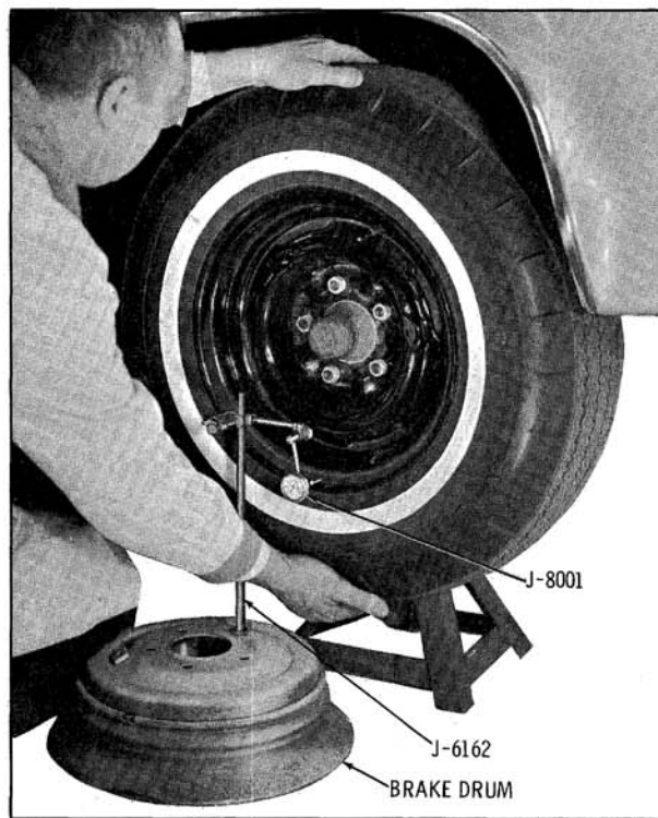
Fig. 9-11 Ball Joint Horizontal Check
