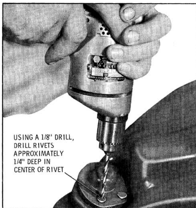
Fig. 9-18A Drilling Ball Joint Attaching Rivets
