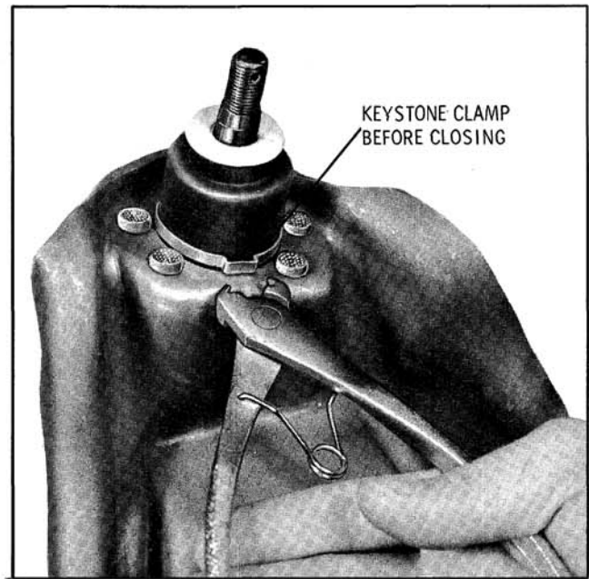
Fig. 9-126 Installing Ball Joint Seal
