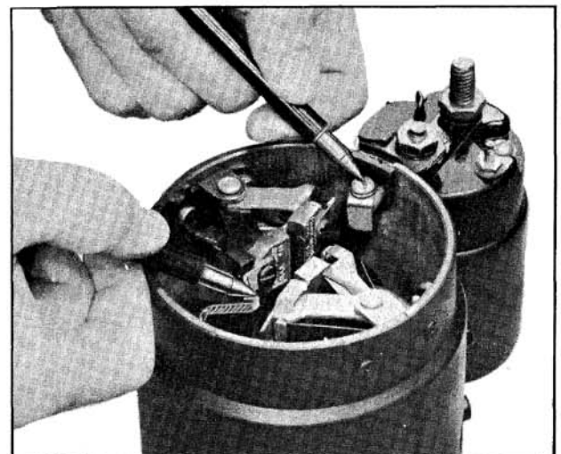
Fig. 13-52 Checking Field Coil for Open
