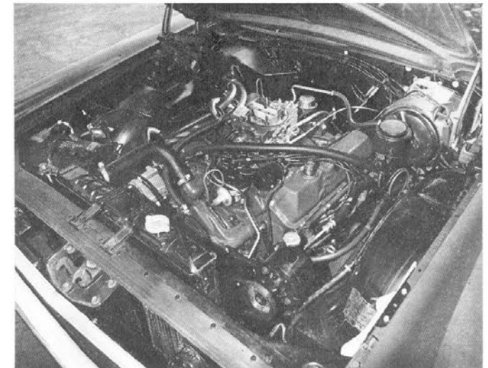
LARGER VALVE covers and big 4-barrel carburetor distinguish 428 engine from others in its family.
