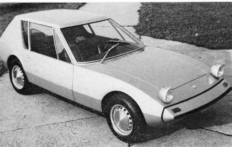
PRINZ CHASSIS, an unusual body style, 106 mph on 55 DIN bhp, add up to NSU's Autonova.
