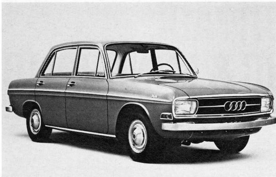
AUTO UNION'S new Audi features four doors and a 4-cycle engine, a new departure from long-time production of the 2-door, 2-stroke/3-cyl. DKW. The new engine has five main bearings, a chain-driven camshaft and pushrods.
