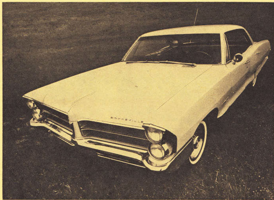
PERFECT EXAMPLE of performance compromise is Pontiac Bonneville, which uses 421-cu. in. engine to drive through long 2.71:1 rear axle.
