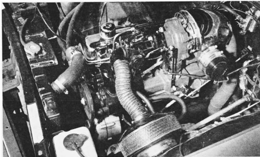
TURBO-SUPERCHARGER was fitted to this Chevelle Six with truck manifold, side-draft carburetor, special adapters and air cleaner relocation.
