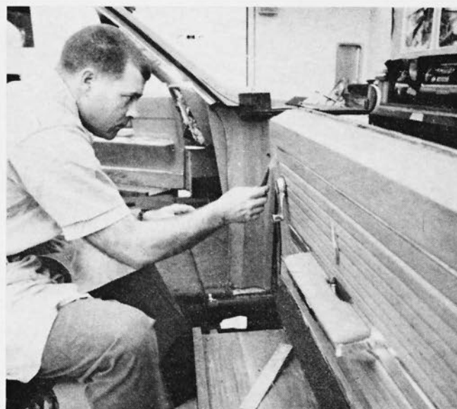
DOOR PANELS are styled, too. Chromed parts are simulated by foil-covering the clay.
