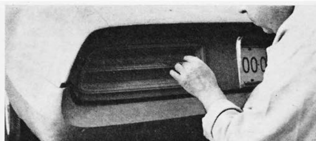
MODELER details stoplights in first full-sized clay version of the Tornado. This design was rejected.
