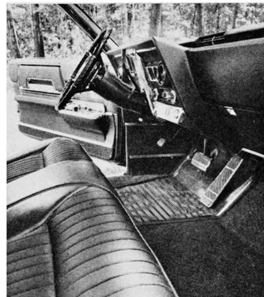
FLAT FLOORS please passengers, but 11-in. drum brakes show alarming fade characteristics.
