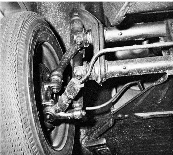
New ball joints replace trailing arm and double grease intervals to 6000 miles.
