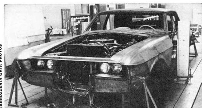
MASSIVE FRONT surrounds Chrysler Street Hemi engine, awaits vertical grille. Headlight wells are to be completely finished around bulbs.
