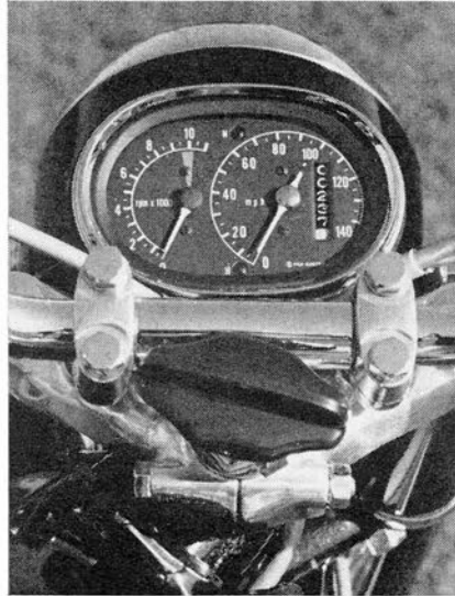
INSTRUMENTS are integrated into the 450's headlamp shell.
