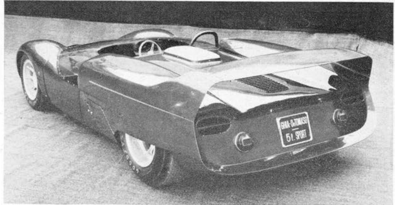
INTENDED FOR competition at Sebring and Le Mans, the Ghia-bodied de Tomaso uses a completely reworked Ford 289-cu. in. engine.
