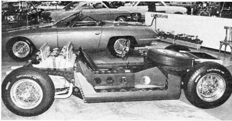
FROM LAMBORGHINI comes a GT prototype car featuring a 244-cu. in. V-12 engine mounted transversely just ahead of the rear wheels.
