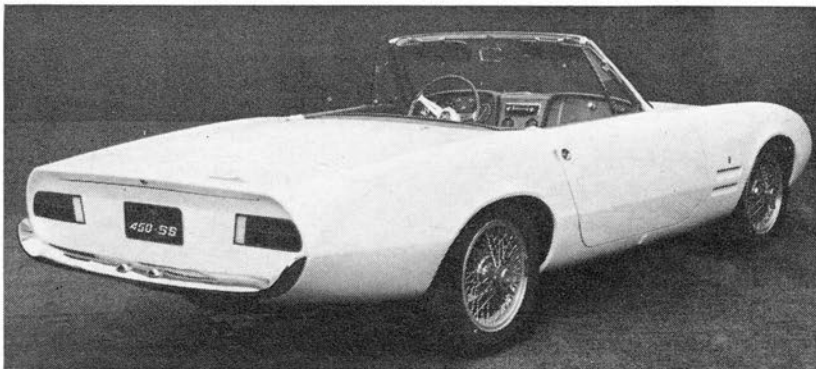
CORPORATION GHIA produces the 450/SS Spyder, a 2+2 sports car on a tubular chassis, using Plymouth's 235-bhp Barracuda S engine.
