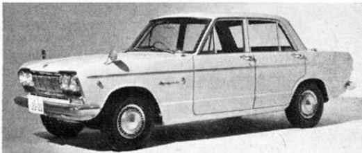
BIG GUN of the Prince line is the Gloria, with an ohc engine and 103-mph top speed.
