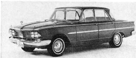
BIG GUN of the Prince line is the Gloria, with an ohc engine and 103-mph top speed.
