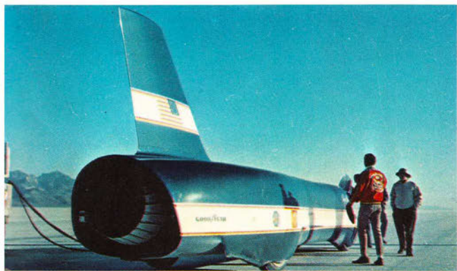
CRAIG BREEDLOVE'S latest jet was built in only 10 months, performed surprisingly well for such a new design. Four wheels support this one and a huge turbo-jet engine propels it. Vertical fin only stabilizes the car, is not used for steering.
