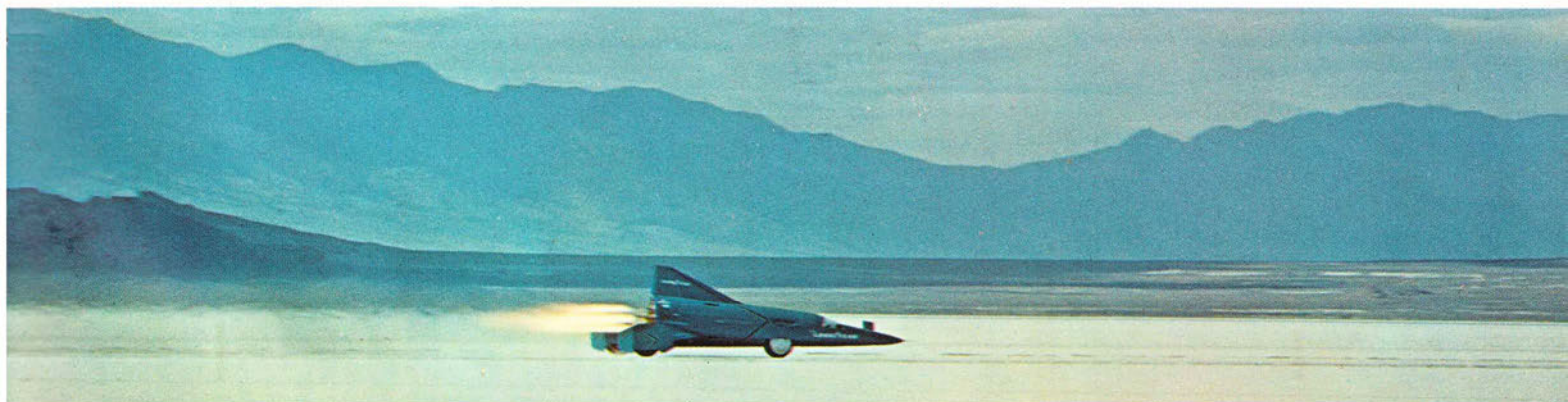
ROCKET CAR built by Walt Arfons was driven by Bob Tatroe (above) on its few spectacular charges across the salt flats (below). Preliminary runs with 15 rockets weren't fast enough so more were added later.
