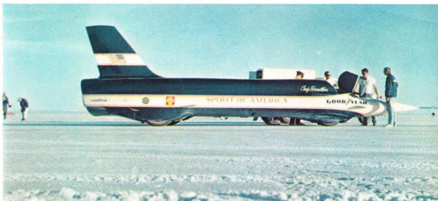
CRAIG BREEDLOVE'S latest jet was built in only 10 months, performed surprisingly well for such a new design. Four wheels support this one and a huge turbo-jet engine propels it. Vertical fin only stabilizes the car, is not used for steering.
