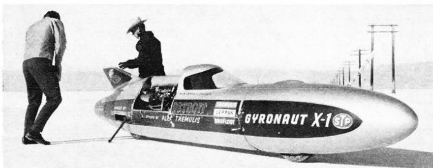
TWIN TRIUMPH motorcycle engines powered the "Gyronaut" on a one-way run of 190.4 mph, but the machine was unable to record the required return.
