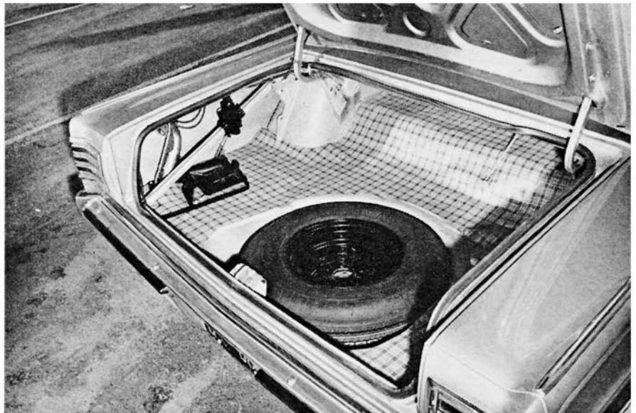
SPARE TIRE fits inside trunk well, leaving broad, nearly flat area for carrying luggage. Jack components are tied down by a spring to keep them from rattling.
