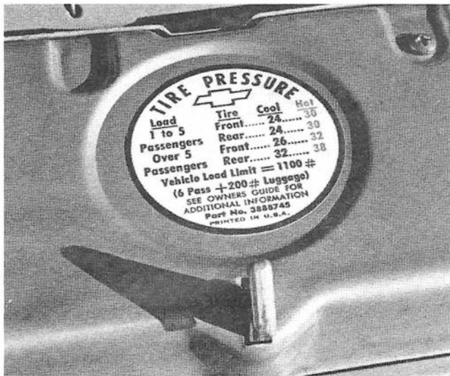
GOOD BIT of customer service is sticker telling recommended tire pressures for various car loads.
