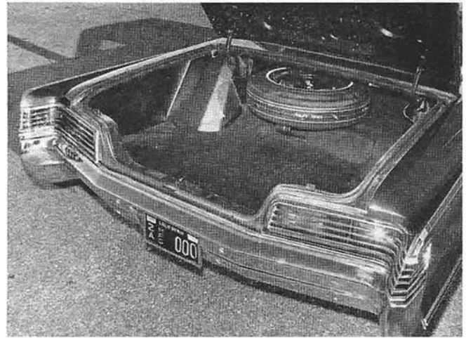
THE 300's luggage compartment, 17.4 cu. ft. in size, is adequate for long-distance touring.
