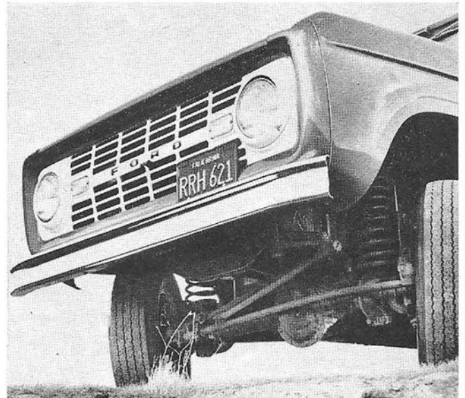
COIL SPRINGS , forged steel radius rods and a 1-in. dia. track bar locate the Bronco's front drive axle.
