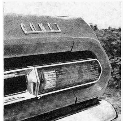
MISFIT panels—here the decklid and taillight sections—typify Comet assembly.
