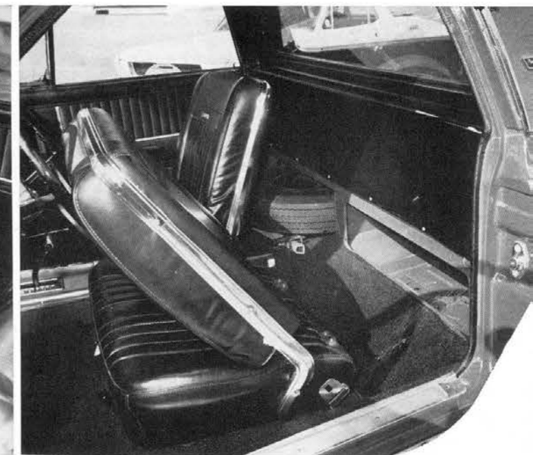
Interior appointments were far above average in both balance and quality. Bucket seats were good compromise between adequate support and softness. Beneath fiberboard panel that finished bulkhead neatly, space was provided for tire, parcels.
