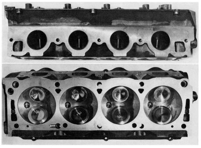
were reduced to .090" locally on the longitudinal centerline. This was done by "clover-leafing" the bore walls on the water jacket side and shifting the water jacket core parting line to the lower end of the bore so that the minimum wall section was placed below the ring travel area. The original four-bolt pattern for attaching the cylinder head was retained and a new head gasket design was employed to seal the high gas pressures.
