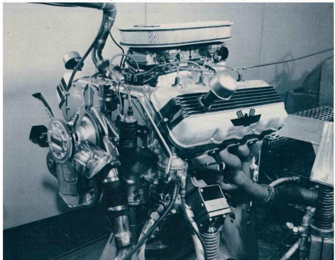
EARLY IN 1962, the Ford 390 engine, which was a modification cubic inch passenger car engine was modified for use as the first of a series of high performance engines. This same basic engine was enlarged by boring to 406 cubic inches later in the year, and to 427 cubic inches in 1963. Refinements in the induction system the overhead camshaft arrangeled to the release of the "High Riser" package. The latest major modification, referred to as the "7,000 rpm Kit," consisted of a valve train change.
