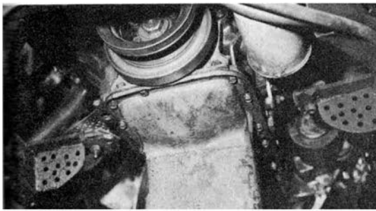
Willys front end clears a deepened oil pan. An FXer must run its tie rod through a sleeved oil pan. Note drilled-out mounts to save weight.
