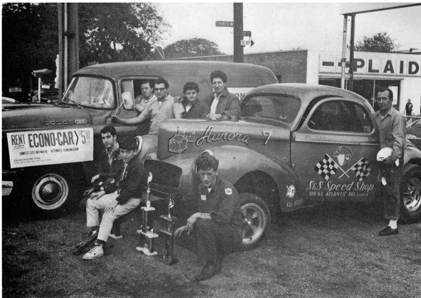
The funny wheelbase Willys is painted to match its ever-present spare parts and fuel truck. The area formerly occupied by a grille now houses an aircraft aluminum fuel filter plus some additional plumbing. The fuel tank mounts above these goodies.
