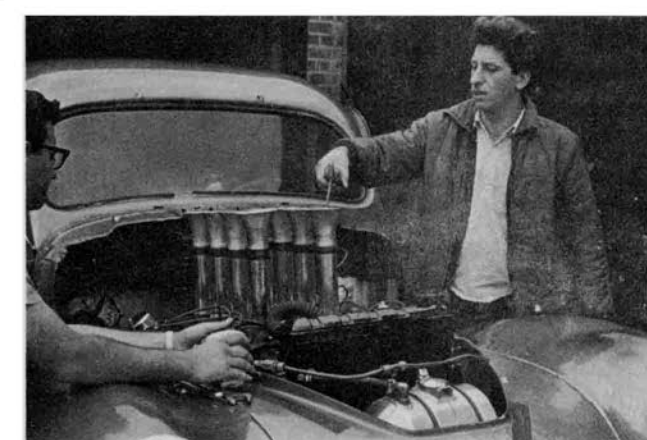
Jerry Lanz primes injectors while driver Joe Black cranks starter. Fuel tank mounts out in front of radiator.
