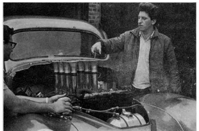
Jerry Lanz primes injectors while driver Joe Black cranks starter. Fuel tank mounts out in front of radiator.
