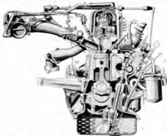
These two views of the 250 SE engine show the fuel injection porting and pump drive, the seven-main-bearing crankshaft, the viscous-drive fan hub, and the single overhead camshaft.
