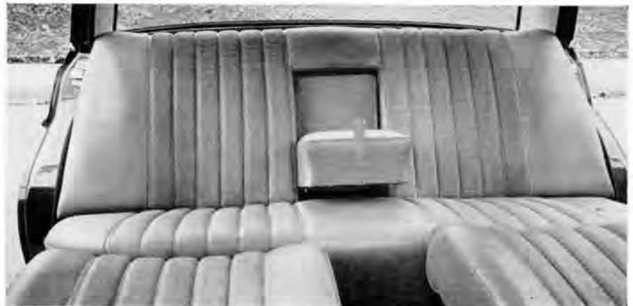
A lay-down driver can bring the front seat back to lock with the rear.
